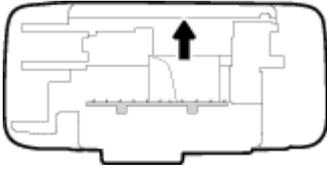
4. Close the cleanout door. Gently push the door towards the printer until both latches snap into place.
