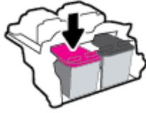
4. Clean the cartridge contacts and printer contacts.
