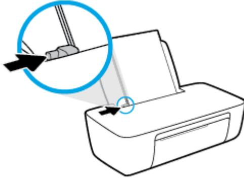
5. Lower the output tray and pull out the output tray extender.
