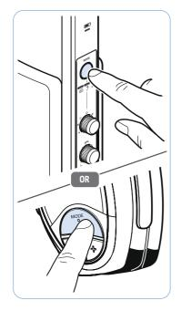
Press the MODE button on the transmitter or on the headphones repeatedly until the additional sound optimization option is activated.
