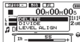
Press the **I◀◀** or **▶▶I** button to open the input level setting pull-up window. Adjust the input level while checking the input sound. (See “Adjusting the input level” on page 39.)
