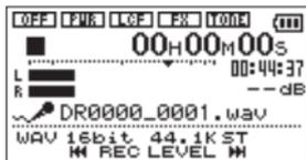
The screen shows the recording file name, the input source, the recording audio file type and sampling frequency. Please confirm that these are as desired before starting recording.
