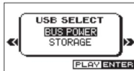
Use the + or – button to select STORAGE, and press the ► button to connect the unit with the computer for data transmission. The message of “USB connected” appears in the display.
