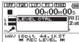
Select **LEVEL CTRL**, and press the ► button to open the level control setting pop-up window.
