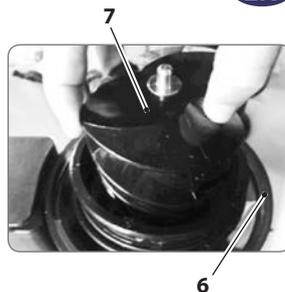
7. Place the cover (8) onto the separator (4).
