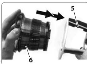
5. Check that the ▼ symbol on the basket (6) needs to align with the triangle mark on the separator (4). Ensure that the basket (6) is completely pushed down.
